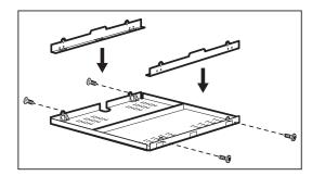
If you use a protection box (an additional accessory 1), the front airflow space of 2 mm and protective floor directly below the appliance are not necessary. You can not use the protection box if you install the appliance above an oven.
